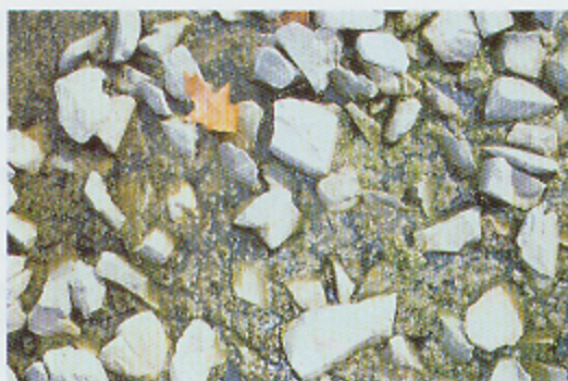
Two rock drains at the Springdale wetland harbor microorganisms that promote manganese removal. Because iron is known to impede manganese uptake and sequestration, the system was designed to remove all iron from the leachate before it enters these drains.
