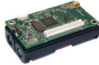
Fig. 8: MICA2 MPR400CB sensor mote [3].
