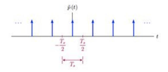
x<sub>a</sub>(t) CAN be totally recovered from impulse-sampled signal x<sub>s</sub>(t)
