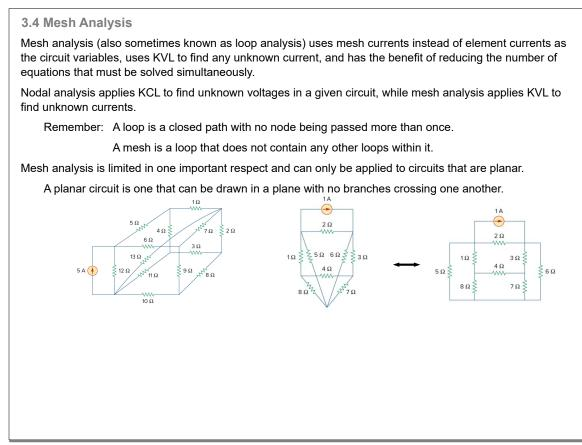
Given a circuit that does not contain current sources and has *n* meshes, mesh analysis is accomplished through the application of 3 steps:
