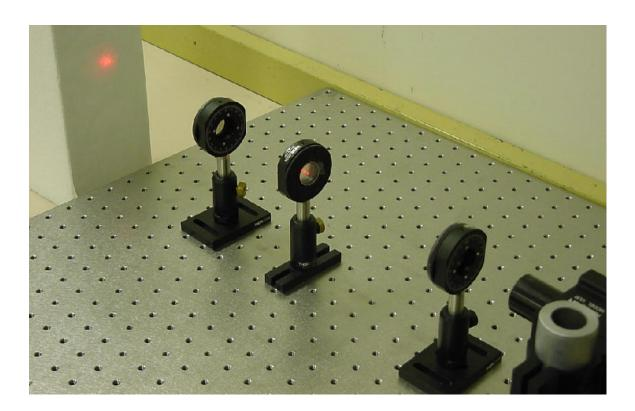
**Fresnel Reflection Equations**: Use a He-Ne laser operating at 632.8 nm, a polarizer, and a power meter to verify Fresnel equations for reflection.
