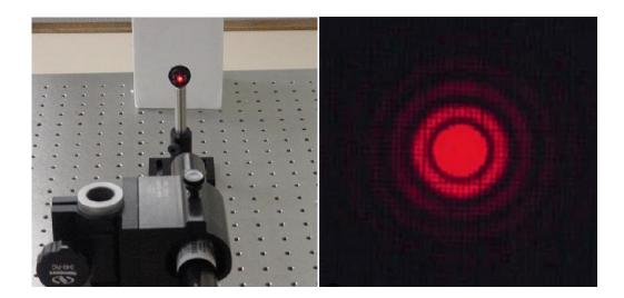
**Transmission Grating**: Reproduce the diffraction pattern shown in the picture by using a helium neon laser operating at 632.8 nm and a diffraction grating. Make all necessary measurements to determine the line spacing.
