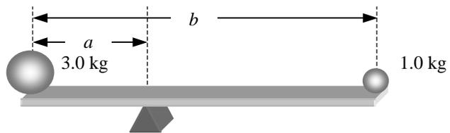
47. Three objects are attached to a *massless* rigid rod that has an axis of rotation as shown. Assuming all of the mass of each object is located at the point shown for each, calculate the moment of inertia of this system.
