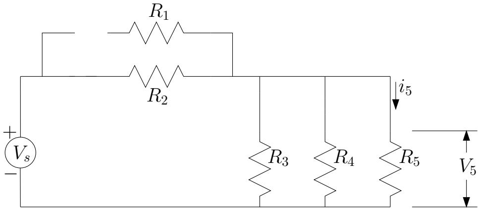
If  $V_s = 5V$  DC,  $R_1 = 1\text{ k}\Omega$ ,  $R_2 = 2\text{ k}\Omega$ ,  $R_3 = 3\text{ k}\Omega$ ,  $R_4 = 4\text{ k}\Omega$ , and  $R_5 = 5\text{ k}\Omega$ , find  $V_5$  and  $i_5$ .
