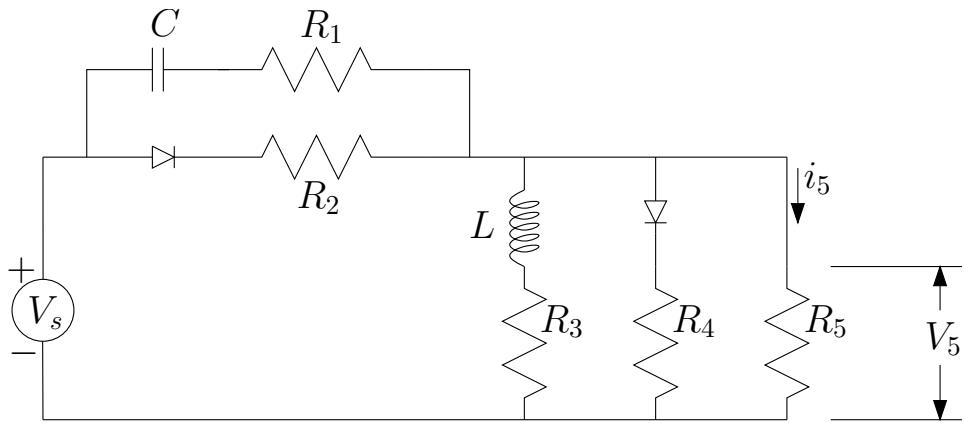
3. (3 points) If  $V_s$  is a DC voltage, draw the equivalent DC circuit.
