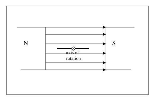
This picture shows the situation when the loop is at the minimum-flux position. When it rotates 90° from this position, the flux is a maximum, as shown in the next picture.
