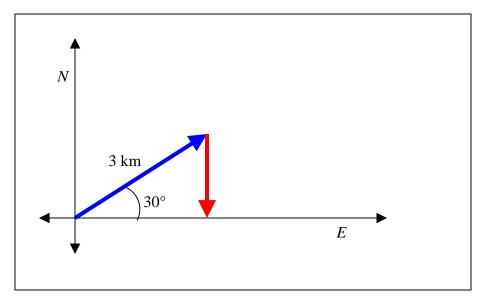
Clearly, the second car will travel due East only. So the collision can only occur when the first car crosses the *East* axis. Thus, the first thing we want to know is where on the *East* axis this will be—let's call that x. From the picture, we see that this will occur at  $x = 3 \text{ km} \times \cos(30^\circ) = 2.6 \text{ km}$ .
