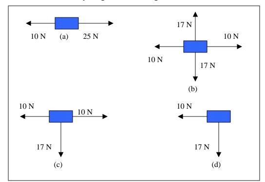
4. Find the magnitude and direction of the net force on the object in each of the free-body diagrams in the figure below.
