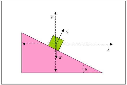
Now, a point on the surface of the incline will necessarily be described by both an x and a y coordinate. All motion along the surface will be 2-d. We've got a big mess on our hands!
