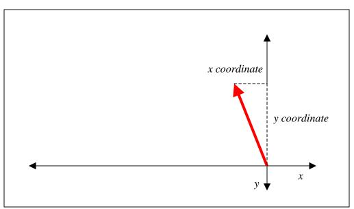
Notice that the x and y coordinates of the final position are precisely the lengths of two legs of a right triangle (dotted lines) and the final displacement vector is the
