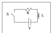
1. In the circuit above, the resistance is  $37\Omega$  and the inductor is 140 mH. After switch S is closed, how long will it be before the voltage difference across the inductor is  $\frac{1}{2}$  V?
