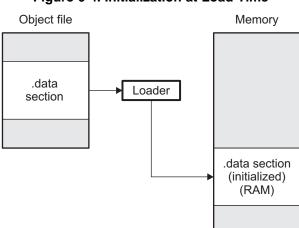
Figure 6-4. Initialization at Load Time
