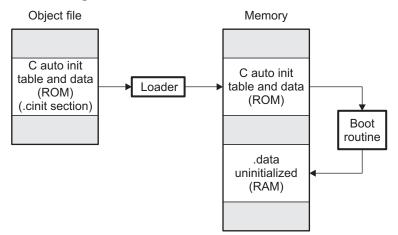
Figure 6-3. Autoinitialization at Run Time
