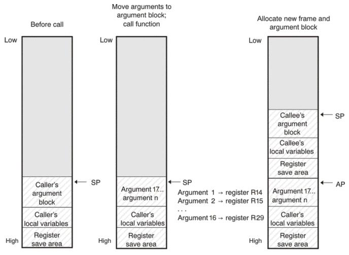
Figure 6-2. Use of the Stack During a Function Call
