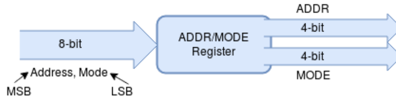
Figure 2.3: The address, mode, & data shared bus scheme
