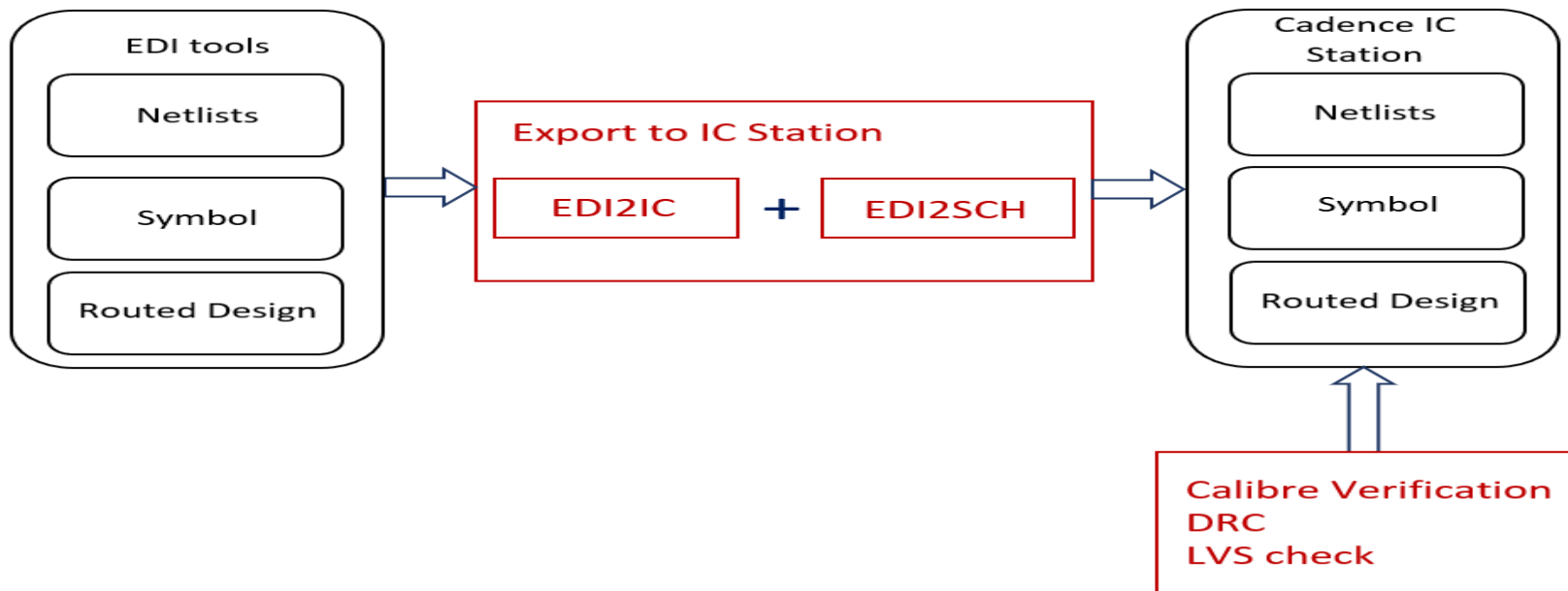
Fig.8 Exporting the design from cadence EDI tools to Cadence IC station
