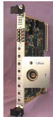
VME ADC, 8 channels (4 pairs), 14-bit differential, pipeline, from SIS/Struck, http://www.struck.de
