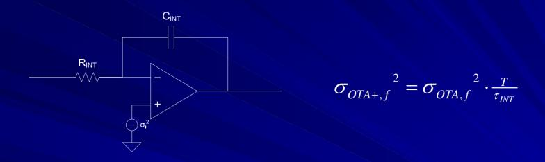
σ<sub>OTA+,f</sub><sup>2</sup> is the continuous-time variance at the output due to 1/f noise in the OTA.
