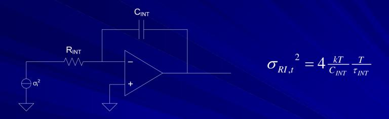
σ<sub>RI,t</sub><sup>2</sup> is the variance sampled onto the integrating capacitor due to thermal noise in the integrating resistor.
